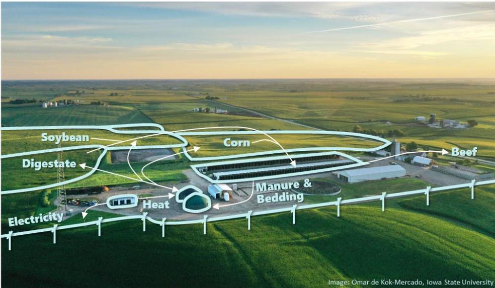
Figure 4. Sievers Family Farms LLC, Stockton, Iowa generates biogas from a diversified crop-livestock system that produces diverse rotations of annual crops and beef. Manure and soiled bedding from cattle barns are mixed with food waste from neighboring industries and anaerobically digested on farm to produce energy that is converted to heat and electricity for on farm use with excess sold to the grid.
